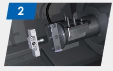
**Connect the AK-1 attachment** Connect the appropriate attachment for your abutment blank to the work material holder of the DWX-42W.
