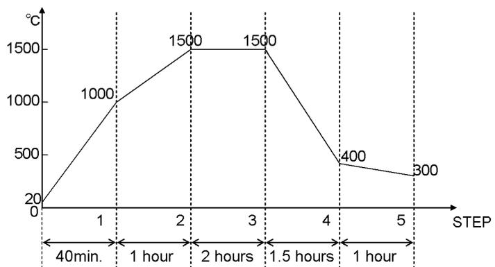
Programmed Start temperature for Zircom speed is 20 °C.
