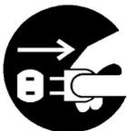
● This mark means forced action and directions to follow as shown inside or around it. The illustration on the left means "Unplug out of power outlet".
